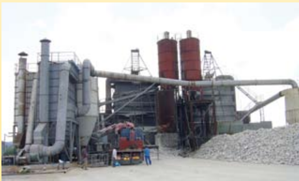
De-dusting of 2 lime stone furnaces. 100 tn/h each
